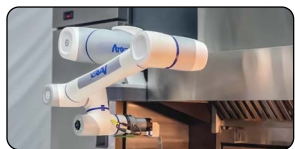
Robotic Arm CR10 – 6-axis co-bot w/ a reach range of 51”+ including an AC100 control panel.
